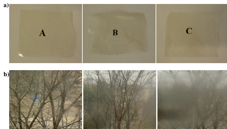
Figure 1. Typical photographs of 30 microns thickness films of A) Carrageenan, B) Carrageenan film containing 5wt.-% of CNW and C) Carrageenan film containing 5wt.-% of cellulose microfibers.
