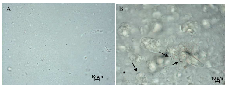
Figure 2. Typical optical micrographs of: (A) Carrageenan with 10 wt.-% glycerol content, (B) carrageenan with 5 wt.-% clay content and 10wt.-% glycerol content. The scale marker is 10 microns in the micrographs.
