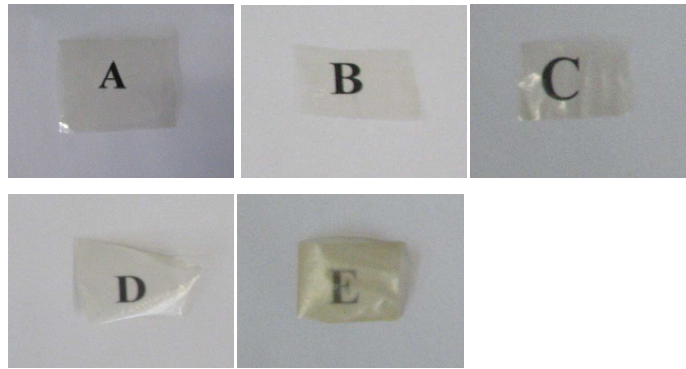
Figure 10. Typical photographs of ca. 30 microns thickness films of plasticized carrageenan containing: A) 0 wt.-% of clay, B) 1 wt.-% of clay, C) 5 wt.-% of clay, D) 10 wt.-% of clay and E) 20 wt.-% of clay.
