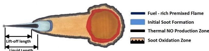
Figure 1. Schematic view of Diesel spray conceptual model proposed by Dec. [6]
