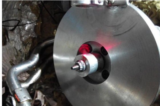
Figure 14: Metal cylinder which replaces the compressor wheel
