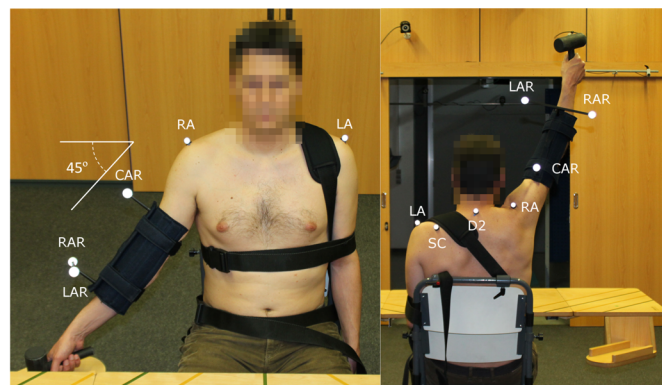
Fig 1. Marker and fastening setup. The image on the left is a front view of the marker setup and trunk fastening. On the right, a rear view of the marker setup and trunk fastening is shown. LA: Left acromion; RA: Right acromion; SC: Medial third of the scapular spine; D2: Second dorsal vertebra; CAR: Central arm; LAR: Left arm; RAR: Right arm.
