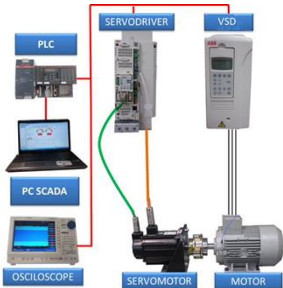
Fig. 4. Test bench components and scheme of connections.
