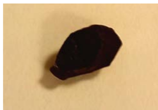
Figure 14. Calcinated hybrid composite-pigment (800 °C, 3h) of the montmorillonite clay modified before adding manganese salt with the surfactant (L9-Mn6).
