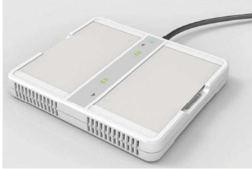
Figura 7. Flat panel Iray Technology (Mars1417V) (IRayTechnology, 2012).
