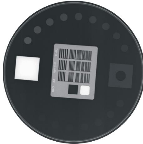
Figura 5. Maniquí TOR 18 FG (Leeds Test Objects, 2015).
