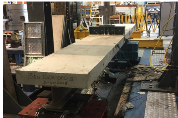
Fig. 2. Composite beam test set-up
