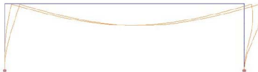
Figure 8 Deformations obtained in the frame without imperfections.
