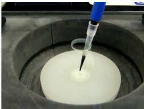
Figure 5.1. Spin-coating process (feeding of dissolved metal solution onto ITO substrate using micropipette).
