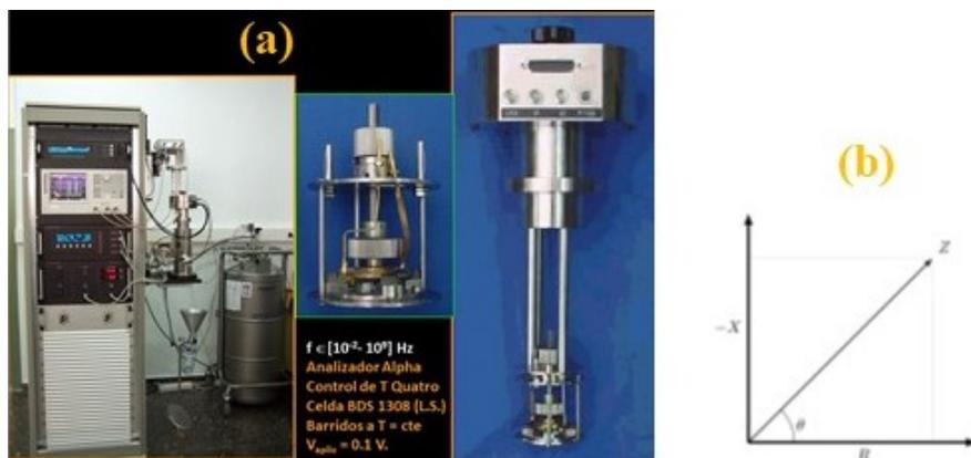
Figure 3.10. (a) Novocontrol Concept 80 set up device and (b) the Complex impedance Cartesian coordinates diagram.
