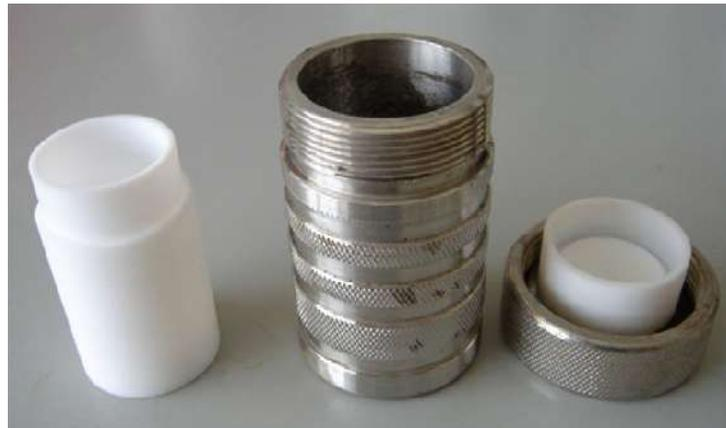
Figure 3.3. A typical Morey autoclaves.
