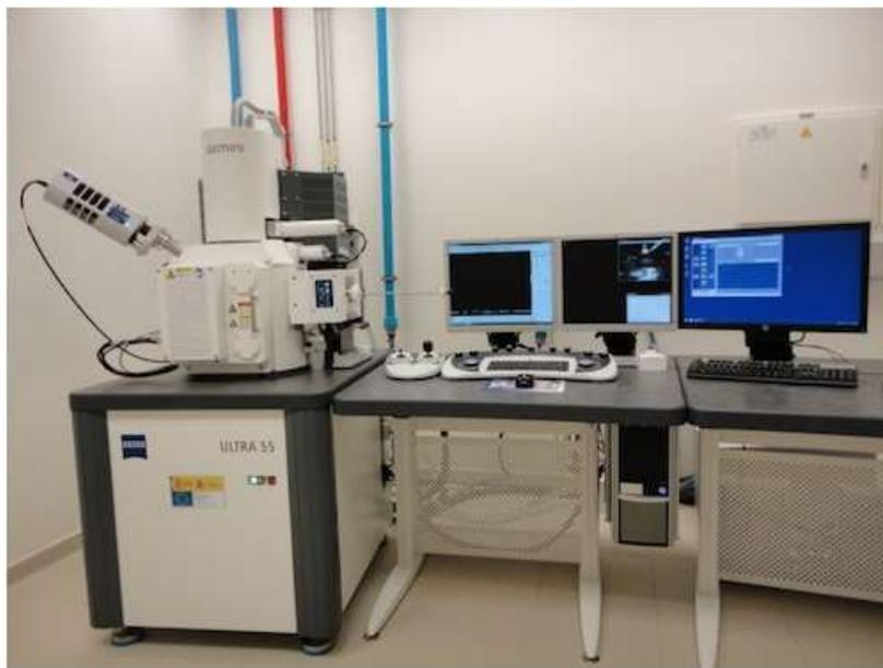
Figure 3.7. image of scanning electron microscopy (FE-SEM), a Zeiss ULTRA 55
