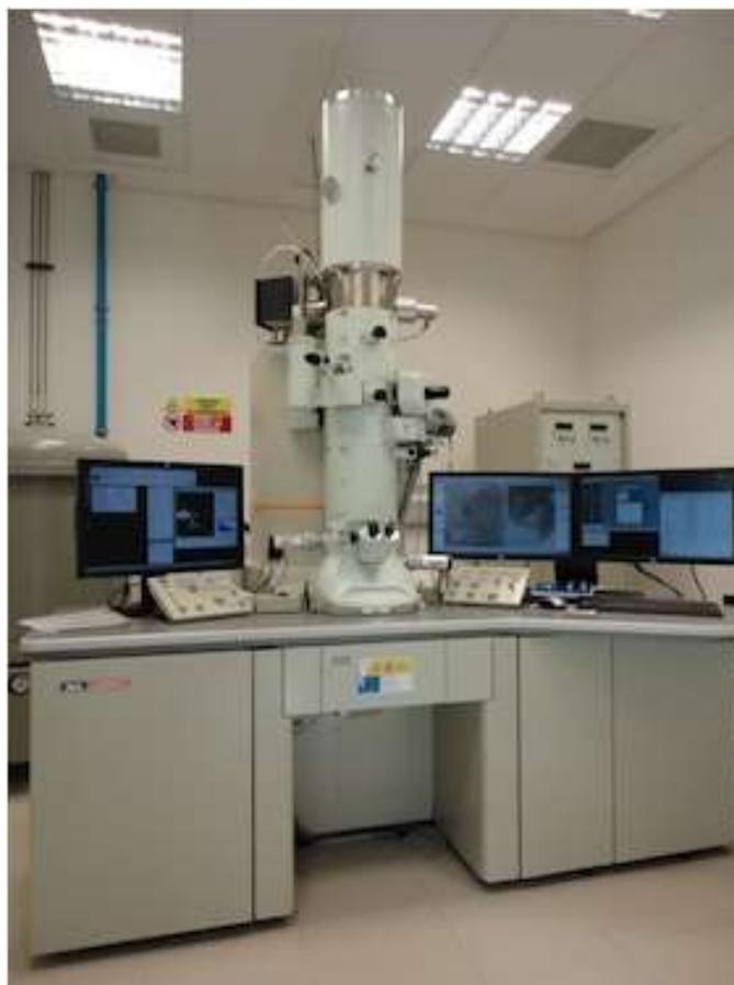
Figure 3.8. image of transmittance electron microscopy (TEM) JEOL JEM 2100F
