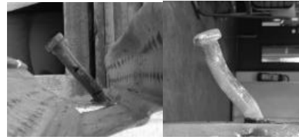
Fig. 2. Plastic deformation of the stud with one and two plastic hinges.
