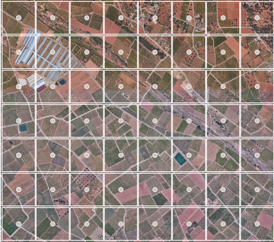
Figure 9.1: Example of a discretized area, calculating the tiles and their center to restrict movements.
