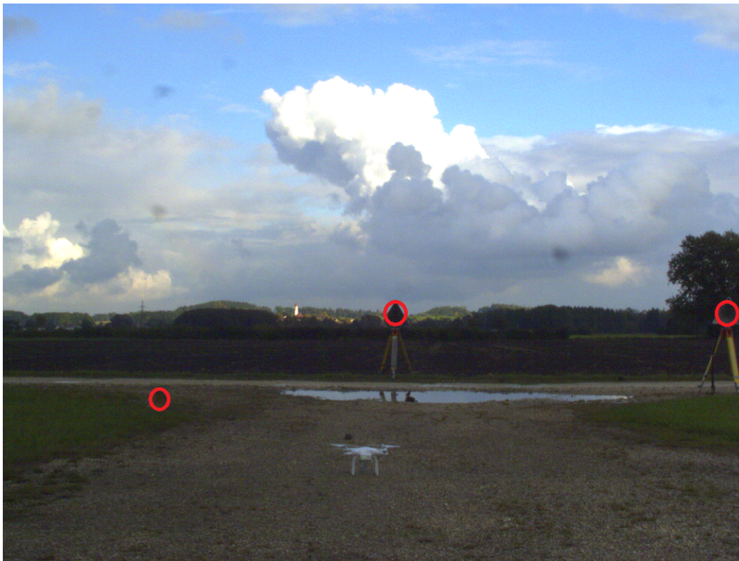
Figure 4.36: Image of the scene with three corner cubes marked with red circles.
