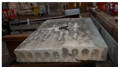
Fig. 9. Failure of slab of SP1A
