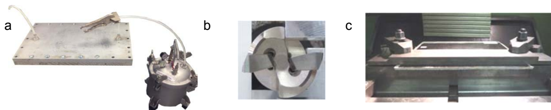
Fig. 1. (a) RTM process; (b) milling tool; (c) fixture in milling machine.
