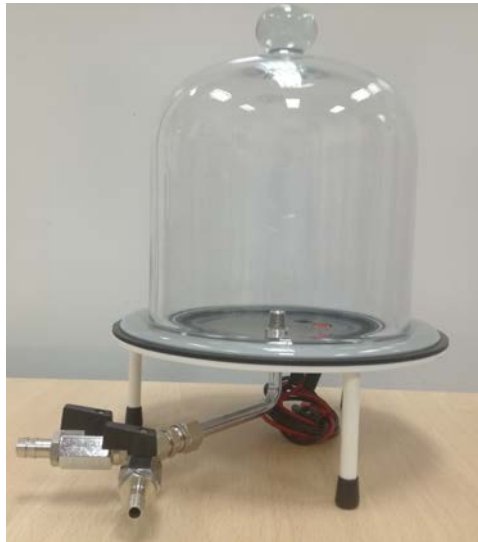
Figure 1. Vacuum pump used to demonstrate the impossibility of sound propagation in vacuum.
