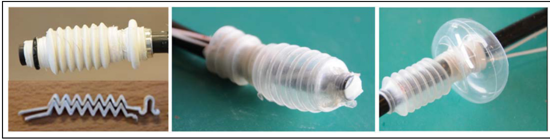
Figure 3. Pneumatic engine mounted on an endoscope model: (left) Previous prototype; (center), current prototype bellows inflated, mobile balloon deflated; (right), current prototype mobile balloon inflated, bellows deflated.
