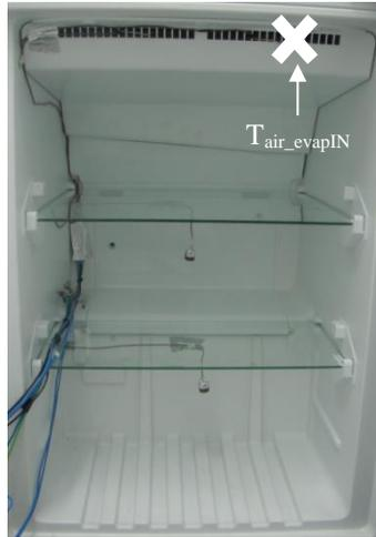
*Figure 56: Air evaporator inlet thermocouple location*
