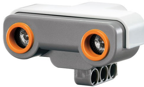
Figure 15 - Lego NXT distance sensor
