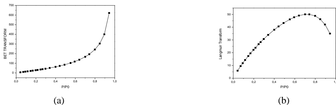
Figure 1: (a)B.E.T. adsorption isotherm and (b) Langmuir adsorption isotherm of natural zeolite
