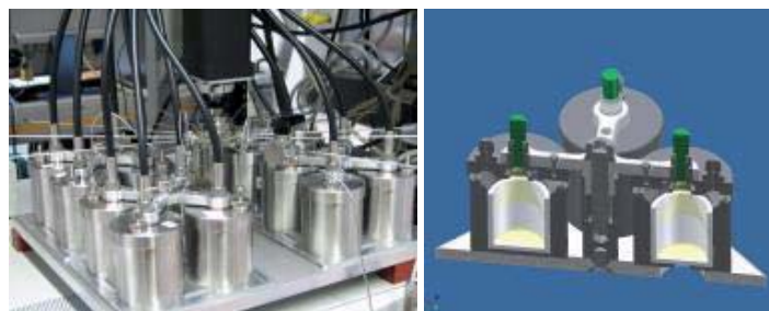
Figure 1. Combinatorial photoreactors applied for gas phase CO 2 reduction.
