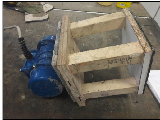
Figure 30. External vibrator VE, producer: Enarco S.A.
