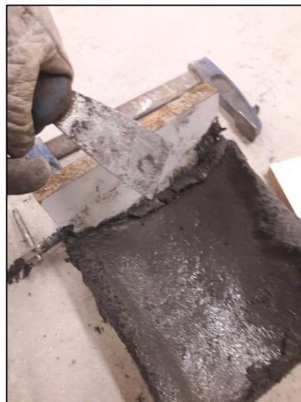
Figure 43. Partially demolding thin shell
