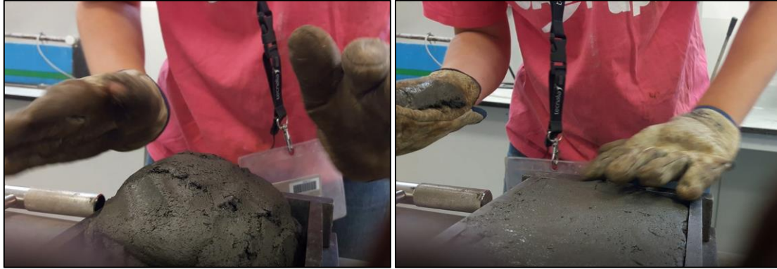
Figure 37. Doughy substance of the concrete a few minutes after mixing (left), and after pushing and removing redundant concrete (right)
