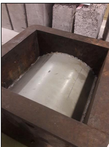
Figure 26. Mold to make negative concrete mold
