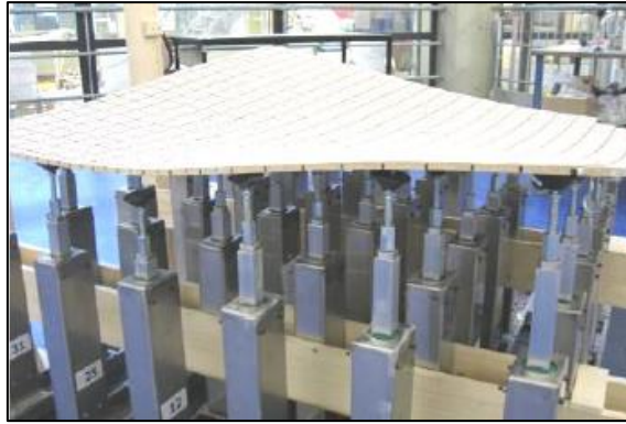
Figure 11. Flexible mold by Rietbergen, Schoofs and Huyghe (2009)
