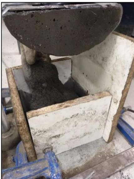
Figure 42. Putting concrete in negative mold
