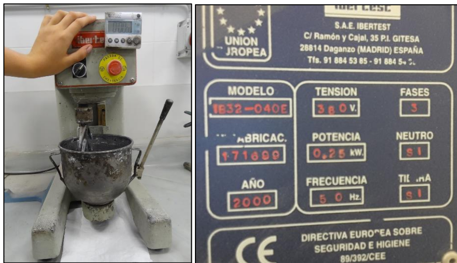
Figure 28. Ibertest mixer 1L (left) and its details (right)
