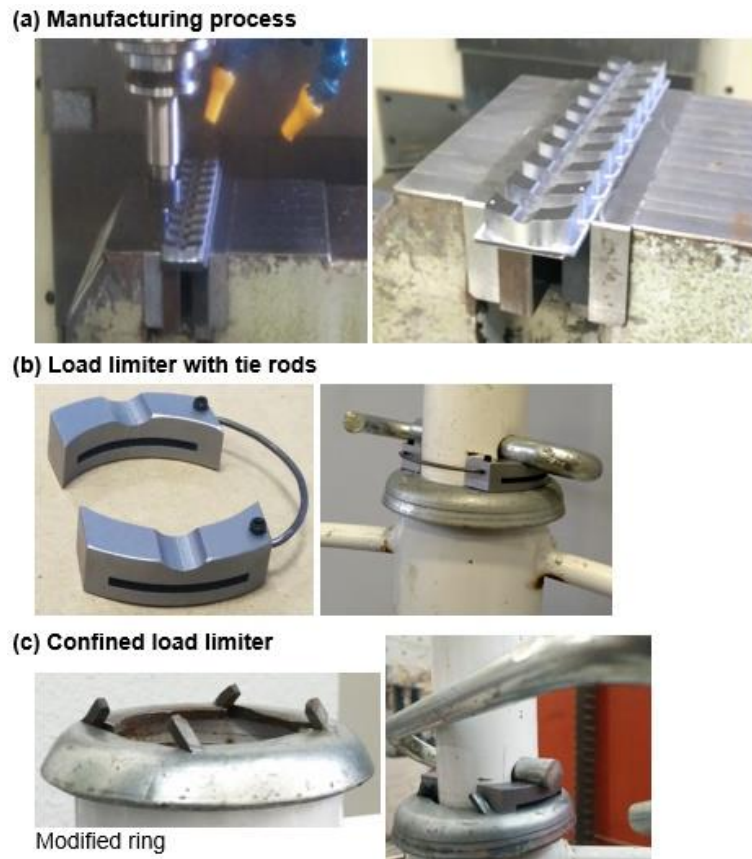
Fig. 6. Production of LL: a) manufacturing process, b) LL with tie rods and c) confined LL.
