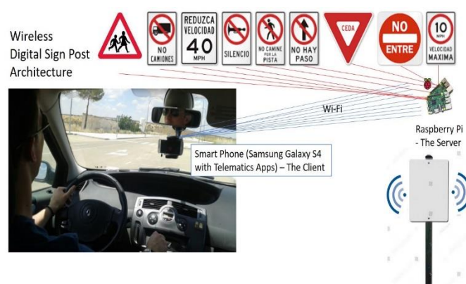
Fig. 3. The programmable Wireless Digital Traffic Sign Post architecture – where the sign post is a server capable of transmitting sign wirelessly to the driver’s client device, which can be the car heads-up displays (HUDs), car dashboard, ADAS display device, or a smart phone.
