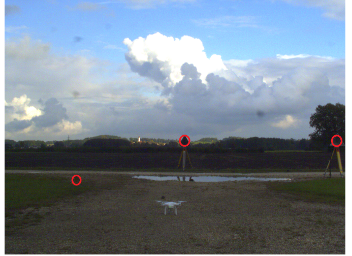
Fig. 10. Image of the scene with three corner cubes marked with red circles.
