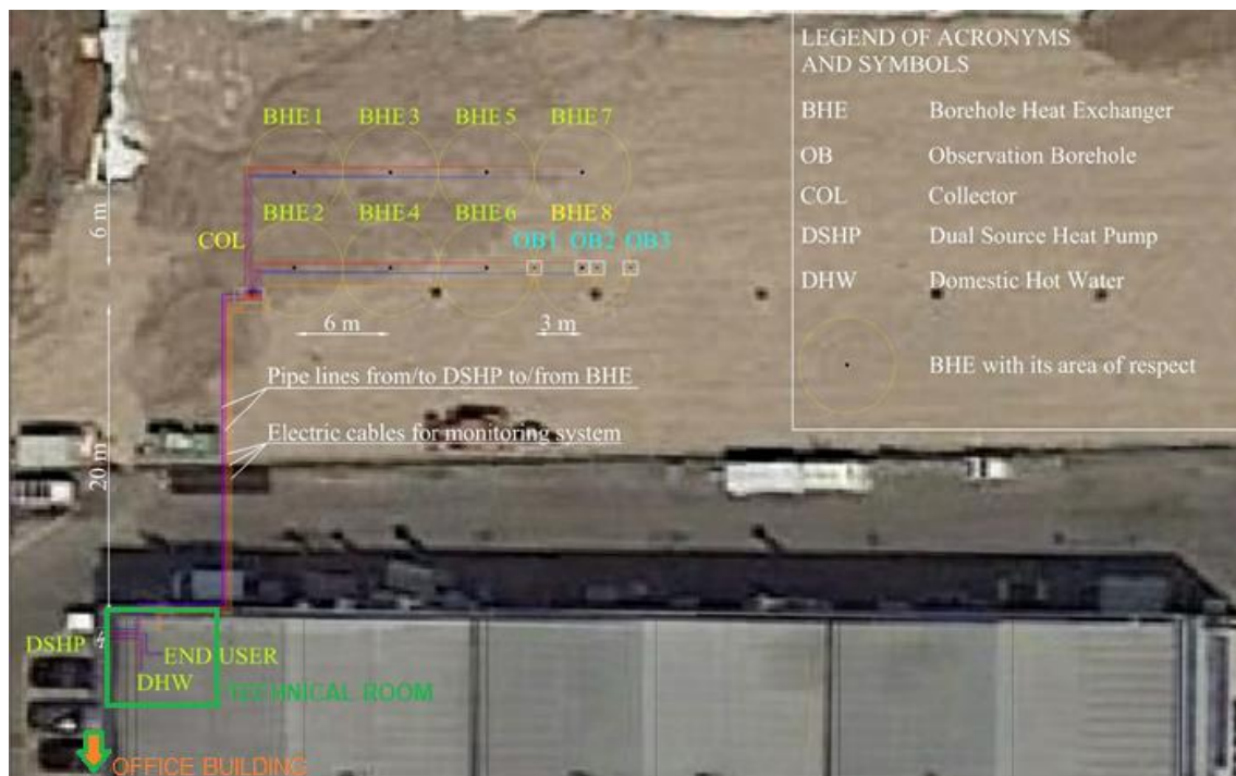
Figure 2.19. Map of the BHE field in the Tribano demo-site. Temperature sensors are located in OB 1, OB 2 and OB 3 (blue), as well as on the head of BHE 8 and COL (yellow) [51]
