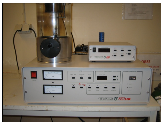
Figure 2. 28. SEM (left) and sputter coater (right) used for analysis in this thesis
