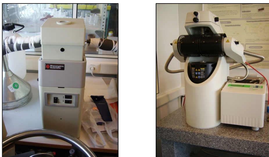
Figure 2. 52. DMTA devices used in this thesis: (left) MarK IV, (right) DMA/SDTA861 e
