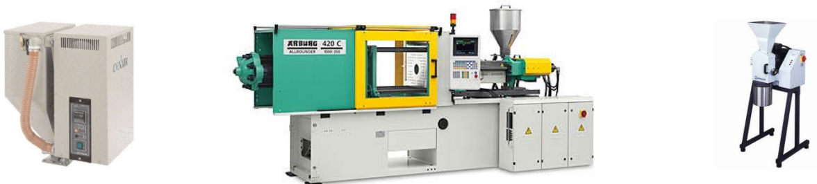
Figure 2. 5. Machinery employed for simulation of reprocessing for both PET and PLA. From left to right: dehumidifier, injector, cutting mill.
