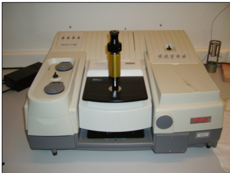
Figure 2. 26. Picture of used IR spectrometer with ATR accessory
