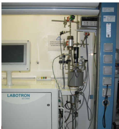
Fig. 2. Microwave reactor and generator
