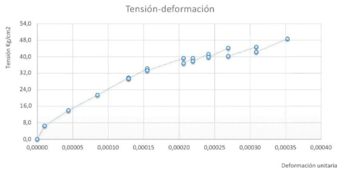
Figure 4. Stress strain curvature, obtained from the flat jack test.
