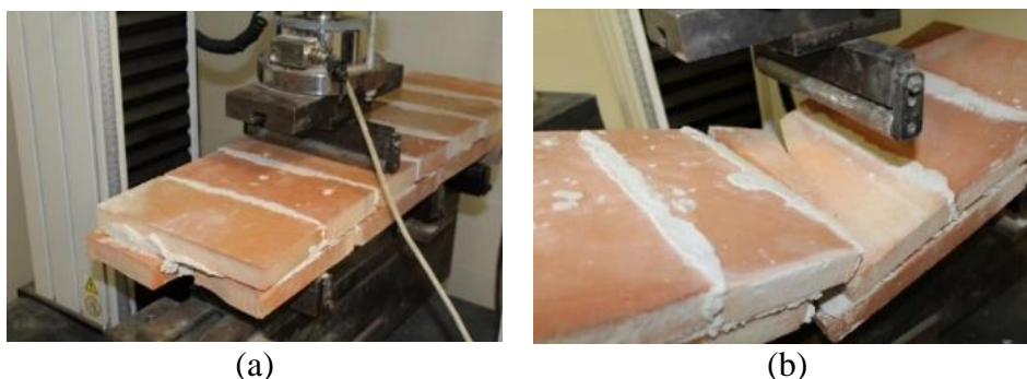
Figure 3. Three points bending test (-a) and failure mechanism (-b).
