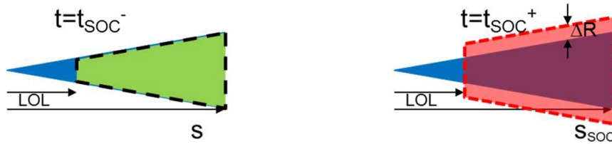
Figure 4 – Schematic showing the simplified inert (left, t=t_{soc-} ) to reacting (right, t=t_{soc+} ) transition as described by the model
