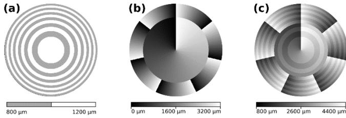
Fig. 1. Design of a multiplexed THz vortex lens. a) Base FZP using (1) with  $p = 1/6$ , b) Multiplexed vortex SPP with topological charges inner part and outer part. c) Composite vortex lens as the superposition of a) and b). Gray levels represent the lens thickness.
