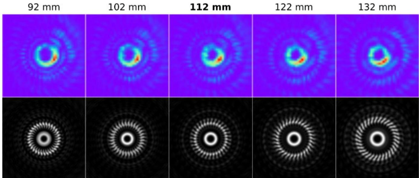
Fig. 3. Experimental results (upper row) and the numerical simulations (lower row) computed using Fresnel-Kirchhoff non-paraxial scalar diffraction theory at different transverse planes around the MVTL focal plane ( $z = 112$  mm).
