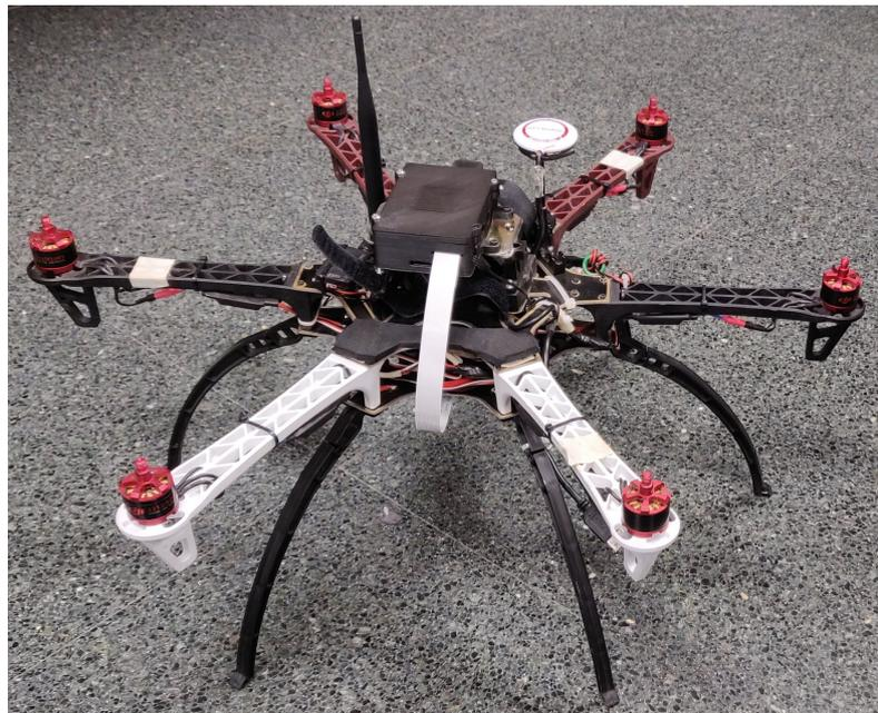
Figure 4. Hexacopter used in our experiments.
