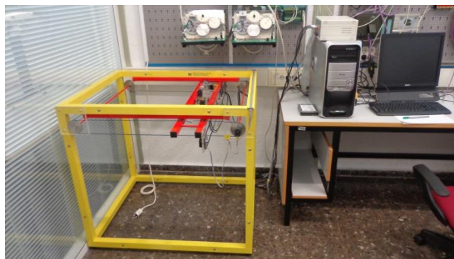
Figure 4. Cartesian robot (3D CRANE module).
