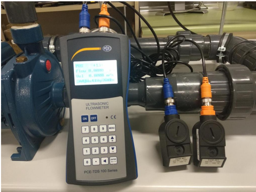
Figure 2. Ultrasound flow meter
