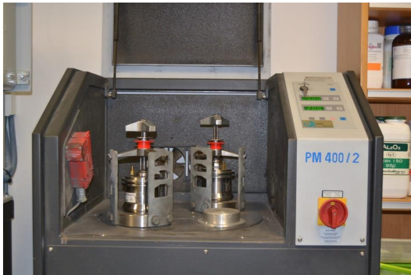
Figure 3.12: Planetary ball milling equipment (Retsch PM 400/2)
