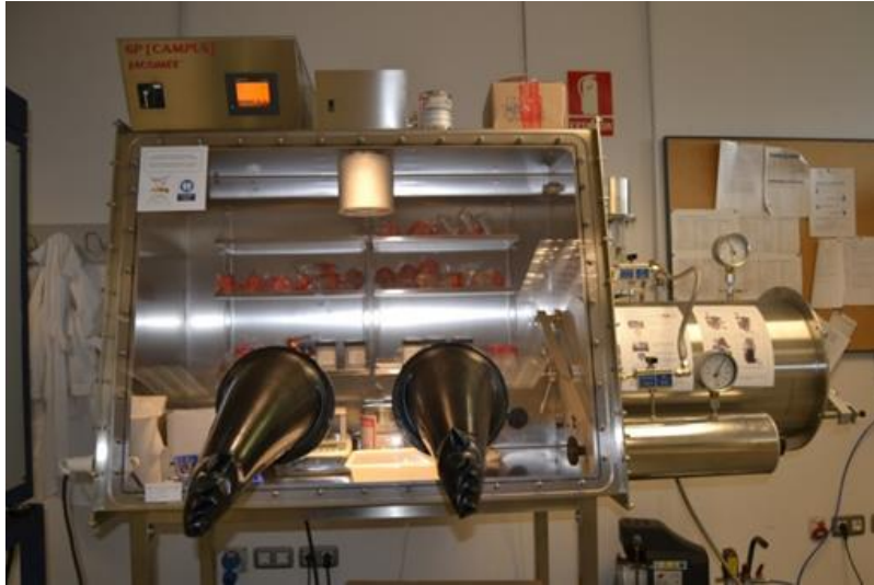
Figure 3.11: Glove box for mixing of powders for compaction
