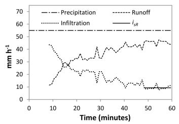
**Figure 2.** Illustrative example of a 1-hour simulated rainfall on a 0.56 m diameter plot at 55 mm h<sup>-1</sup> rainfall intensity. The infiltration curve was drawn by subtracting the runoff rate from the intensity. The experimental steady-state infiltration rate,  $i_{sR}$  (9.3 mm h<sup>-1</sup>), was estimated considering the last thirteen data points
