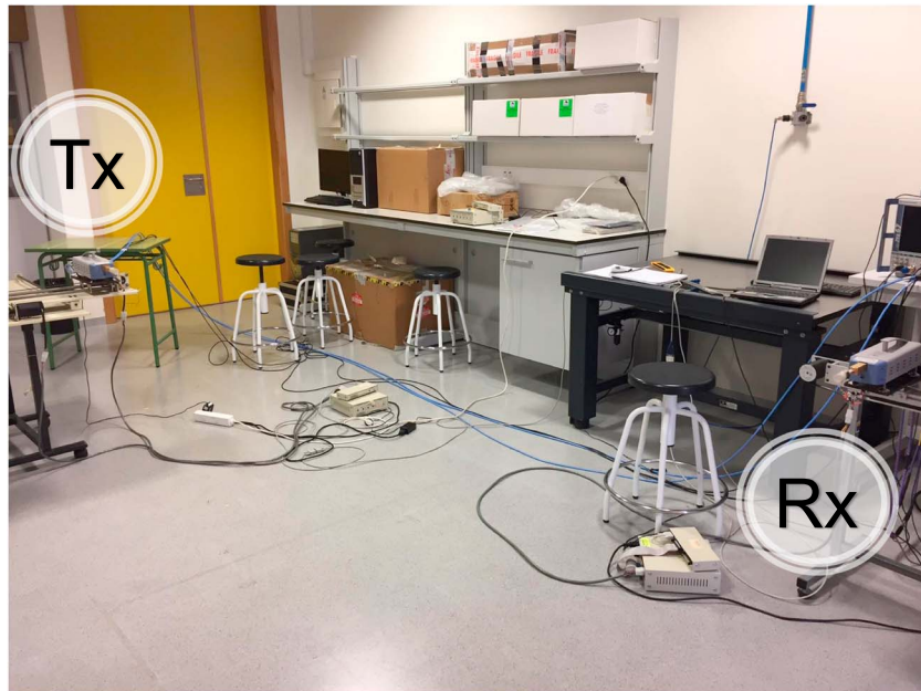
Figure 1. Lab with Tx and Rx antennas and positioners.
