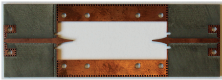
Fig. 3. Manufactured back-to-back transition without top and bottom covers
