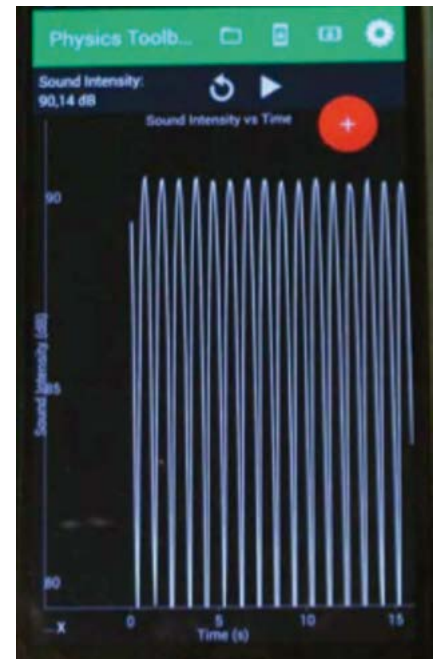
Figure 4. Variations of the sound level of the acoustic beat as shown on the smartphone's screen by the application Physics Toolbox Sound Meter .
