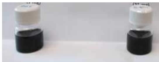
Figure S12. Inks prepared with B(G) (left) and f -B(G) 2 (right) in DMF (1 mg/mL).
