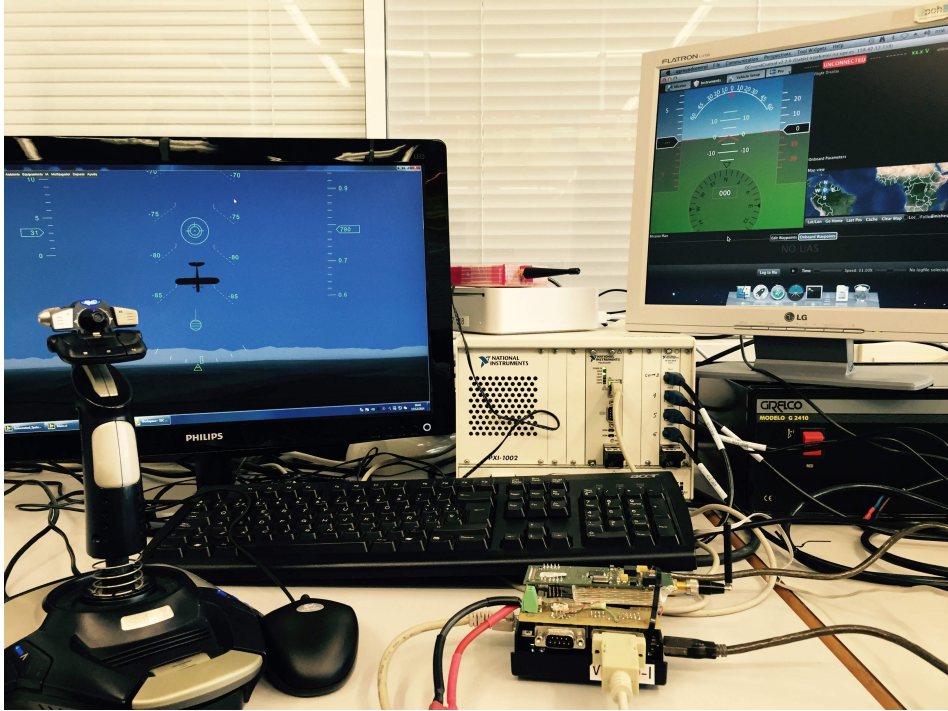
Figure 4.1. Hardware in the loop simulations setup
