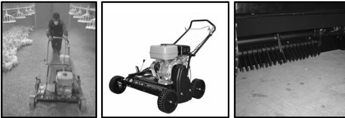
Figure 2: Machine used for litter aeration and detail of the rotative parts
