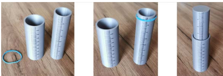
Fig. 1 Left: Archie's smaller and larger cylinders along with a small rubber band. Center: The rubber band wrapped around the top of the smaller cylinder. Right: An Archie with a volume set to 140 ml.
