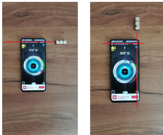
Fig. 1 Left: The magnet is moved next to the right side of the smartphone until the smartphone shows north to be to the right. Right: The magnet is moved above the upper edge of the smartphone until it shows north to be up. The location of the magnetometer is where the right and upper directions intersect.
