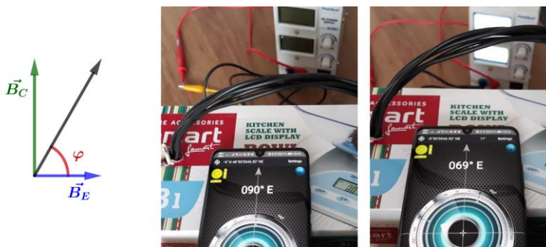
Fig. 5. Left: The addition of the magnetic fields of earth and the coil. Center: The setup of the compass at a 90^\circ angle to the magnetic field of the coil. Right: The change of the angle when current is flowing through the coil.
