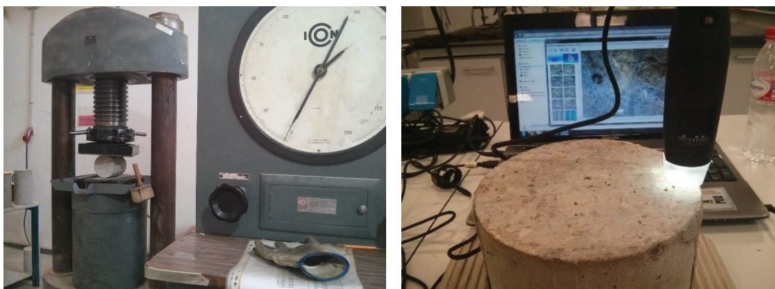
Figure 1. Precracking by splitting test (left) and USB microscope to analyze cracks (right).
