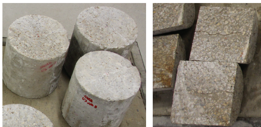
Figure 10. Surface cracks healed in specimens with large cracks healing under WD cycles, and internal crack after cutting the cylinder transversally to the crack.
