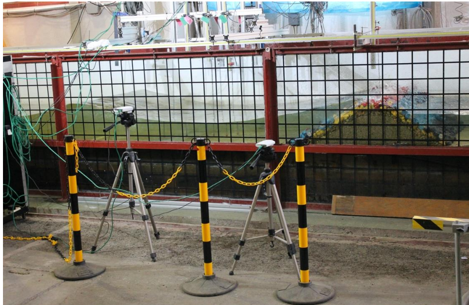
Fig. 3.12. Video cameras recording the physical tests.
