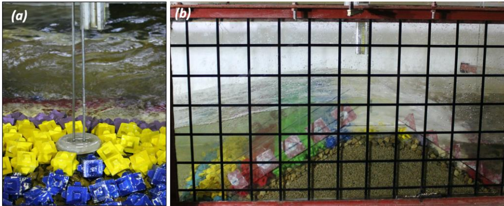
Fig. 3. 9. Overtopping layer thickness (OLT) measurement: (a) wave gauge S10, and (b) visual inspection of OLT.
