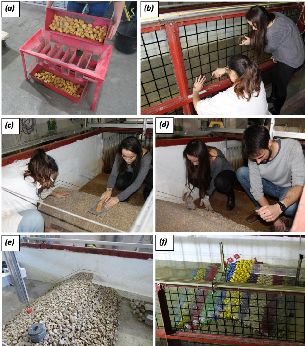
Fig. 3. 7. Construction process: (a) characterization of the materials, (b) drawing the cross section, (c) construction of core, (d) construction of filter, (e) view of the model with core, filter and tube for S10 gauge, and (f) Cubipod®-1L physical model.
