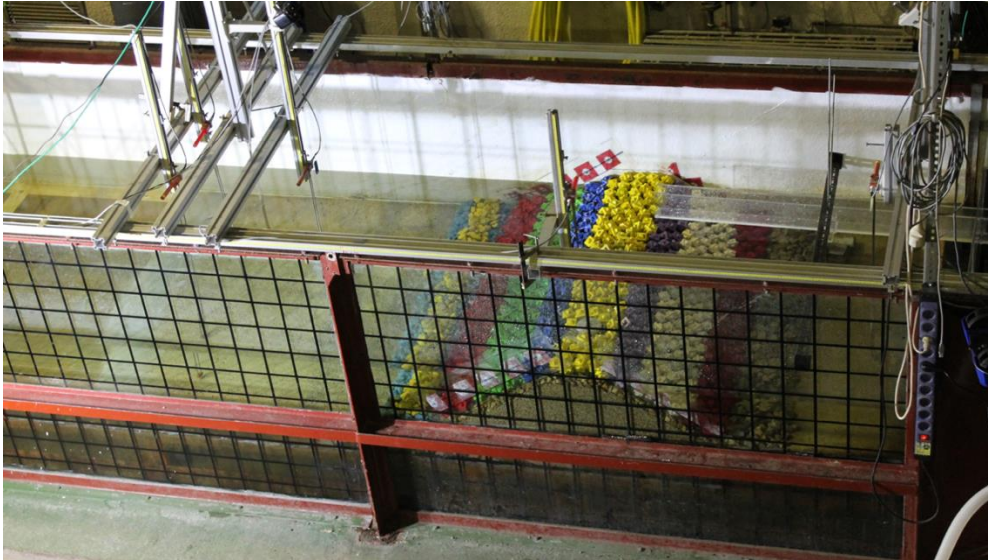
Figure 3. Experimental set up with the Cubipod®-1L armored breakwater model.
