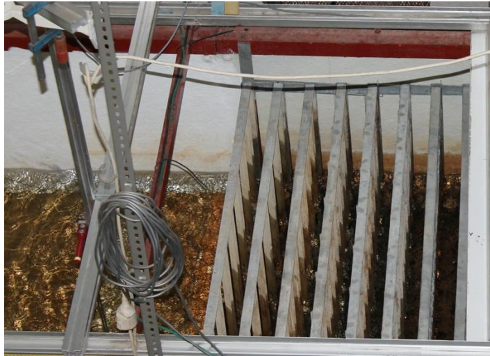
Fig. 3. 2. Passive wave attenuator.
