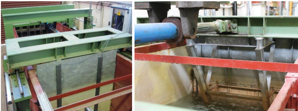
Fig. 3. 3. Piston-type wavemaker of the LPC-UPV wave flume.
