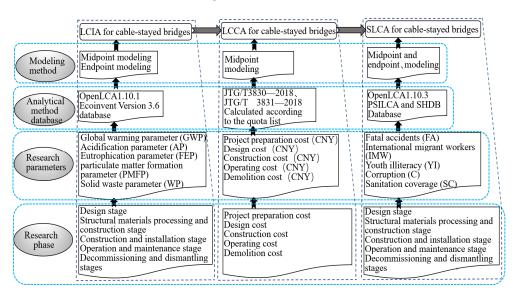
Figure 2. Schematic diagram of the LCIA, LCCA, and SILA analysis process.
