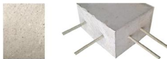
Figure 1. Lime Concrete + GFRP bar.
