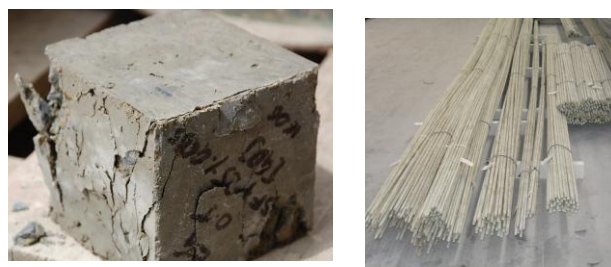
Figure 16. a: Lime Concrete – b: GFRP bars
