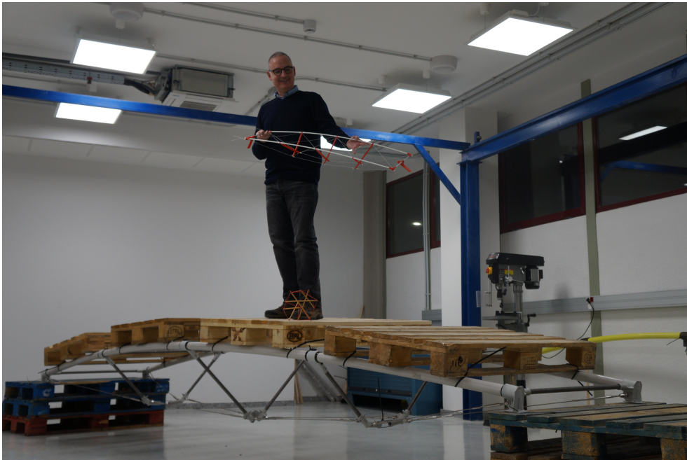
Figure 94: The experimental footbridge prototype in service.
