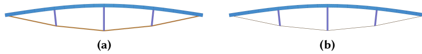
Figure 50: Configurations with the same rod slenderness \bar{\lambda} = 1.5 and different cable-rod slenderness ratios: a) \bar{\lambda}_c/\bar{\lambda} = 5 and b) \bar{\lambda}_c/\bar{\lambda} = 15 .
