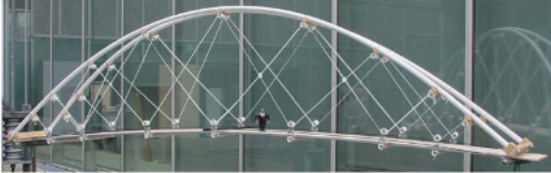
(b) Conceptual model of a prestressed composite footbridge [26].
