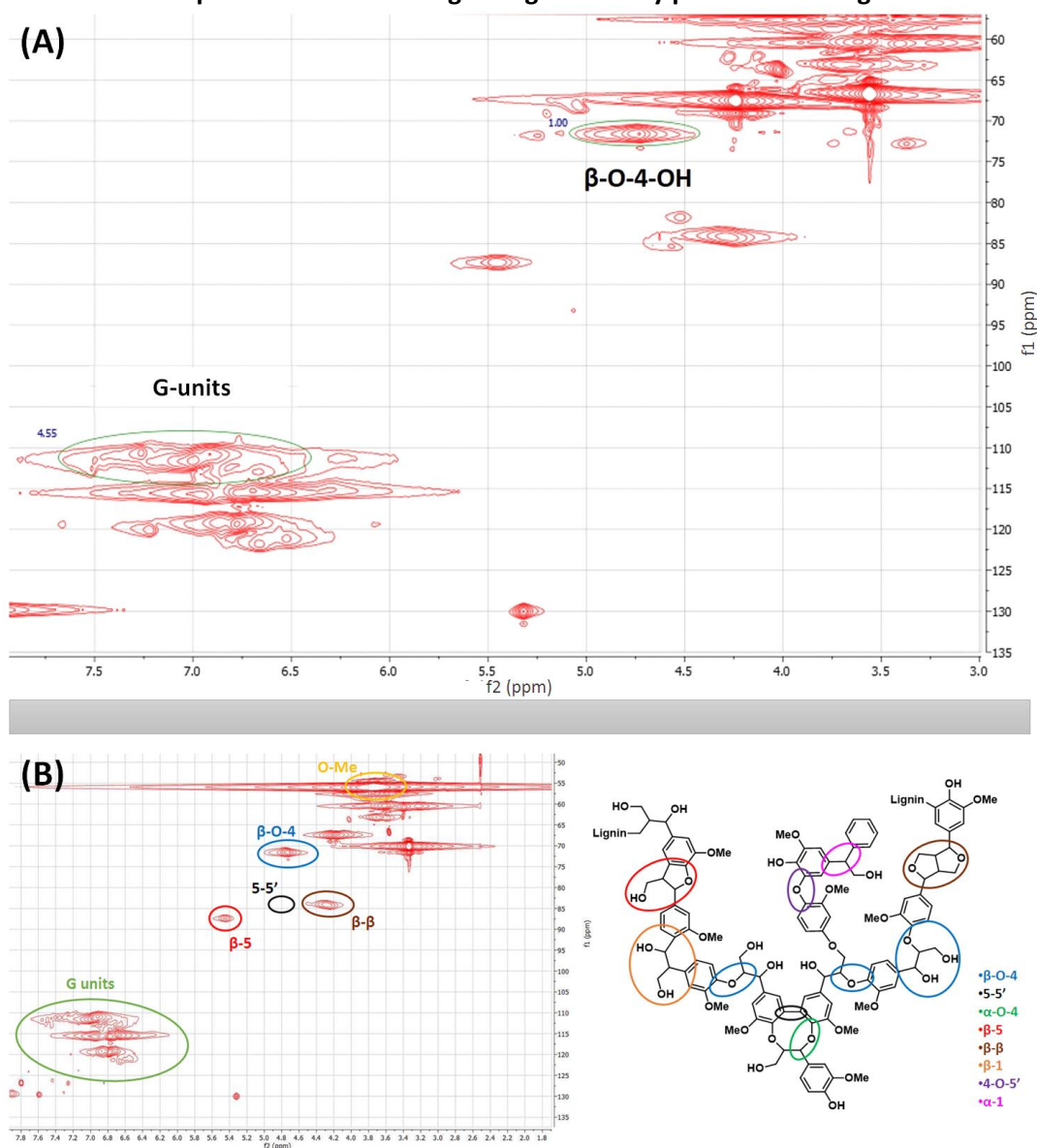
Figure 2. (A) Example of 2D ^1\text{H} - ^{13}\text{C} HSQC NMR spectra of the technical lignin extracted from pinewood by acidolysis using a dioxane/water blend (90/10 v/v) and 0.2 M of HCl, and (B) Identification of main aliphatic interconnecting linkages natively present in the lignin.
